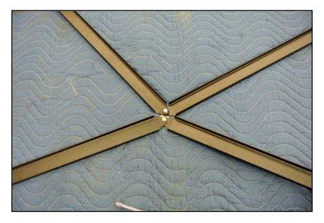
Repeat for the other Pem stud on bracket. Invert the assembly and mount to the four corners of the top of upper frame of the game (2 persons are recommended to perform this part) using ½-20x3/4" carriage bolts (2) on front of game (see below),
