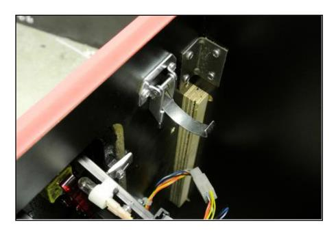
Once released, lift the console lid to open. The wire harness connecting the front console to the main body has multiple connections. The connectors for optical sensors are labeled A, and B. The connectors are such that no accidental mismatching should occur. Power is run through a separate hole in the console.
