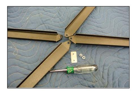
Place canopy connection bracket so that the PEM studs stick up through two brackets on the left, and two on the right. Use an 8-32 nut with captive star washer to secure brackets on stud (see below).
